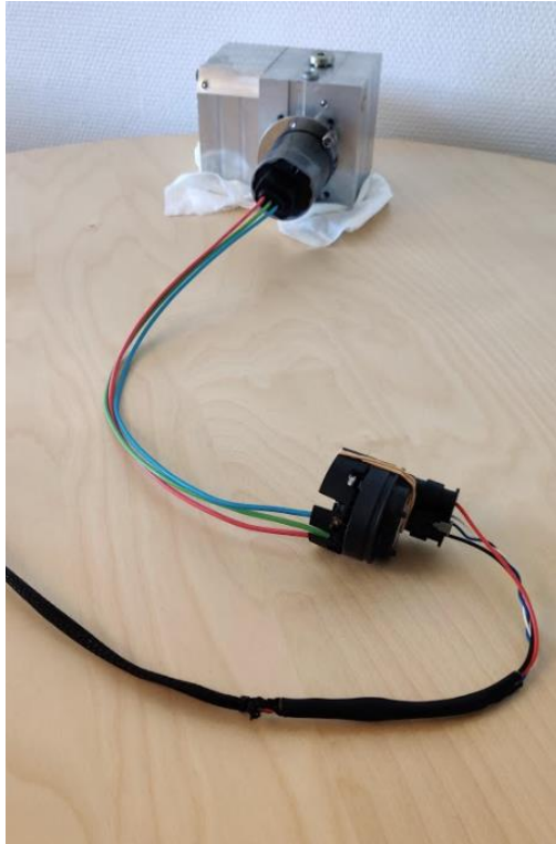
Figure 3-2: ECU connected to actuator and pump block.
