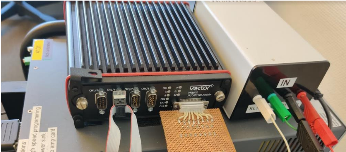
Figure 2-6: VN8970 System with power supply.
