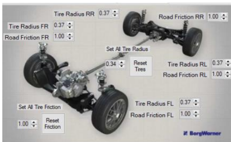
Figure 2-4: Panel that can change road friction coefficients.
